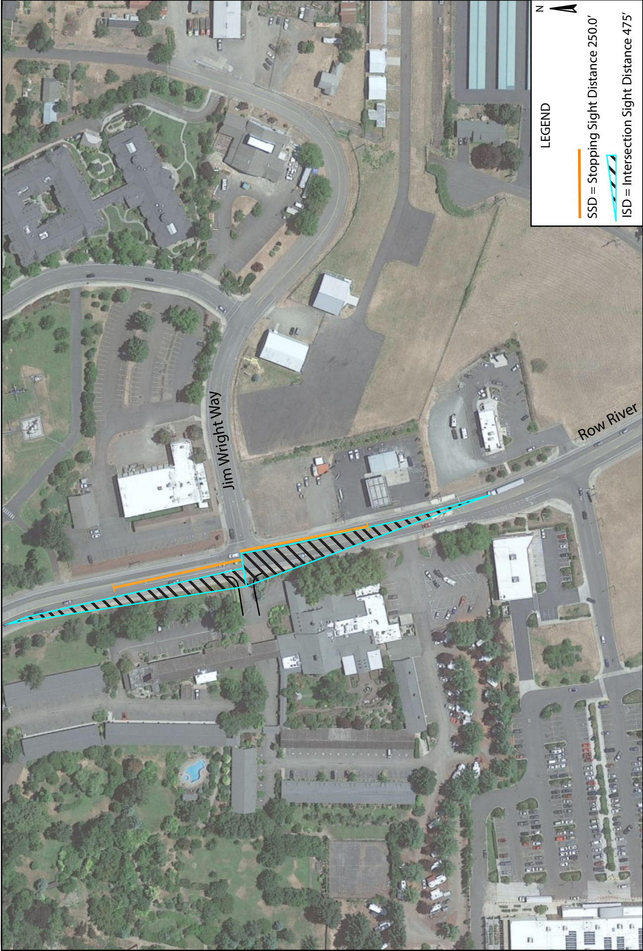
Figure 11: Intersection and Stopping Sight Distance North Access
