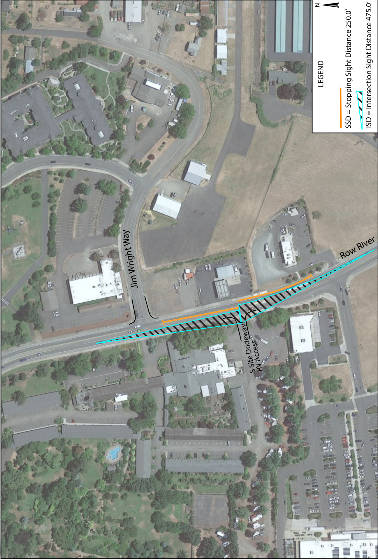
Figure 12: Intersection and Stopping Sight Distance South Access
