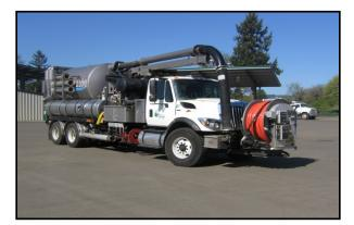
Vactor truck used to vacuum and/or jet sanitary sewer lines, manholes, storm drainage facilities, and excavation sites.
