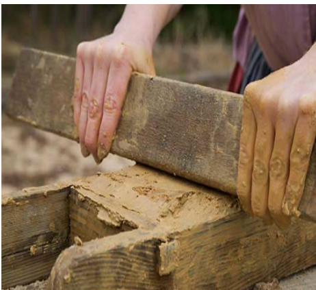
Figure 1. Forming Terra Cotta Unit ( www.history.org/almanack/life/trades/tradebri.cfm )
