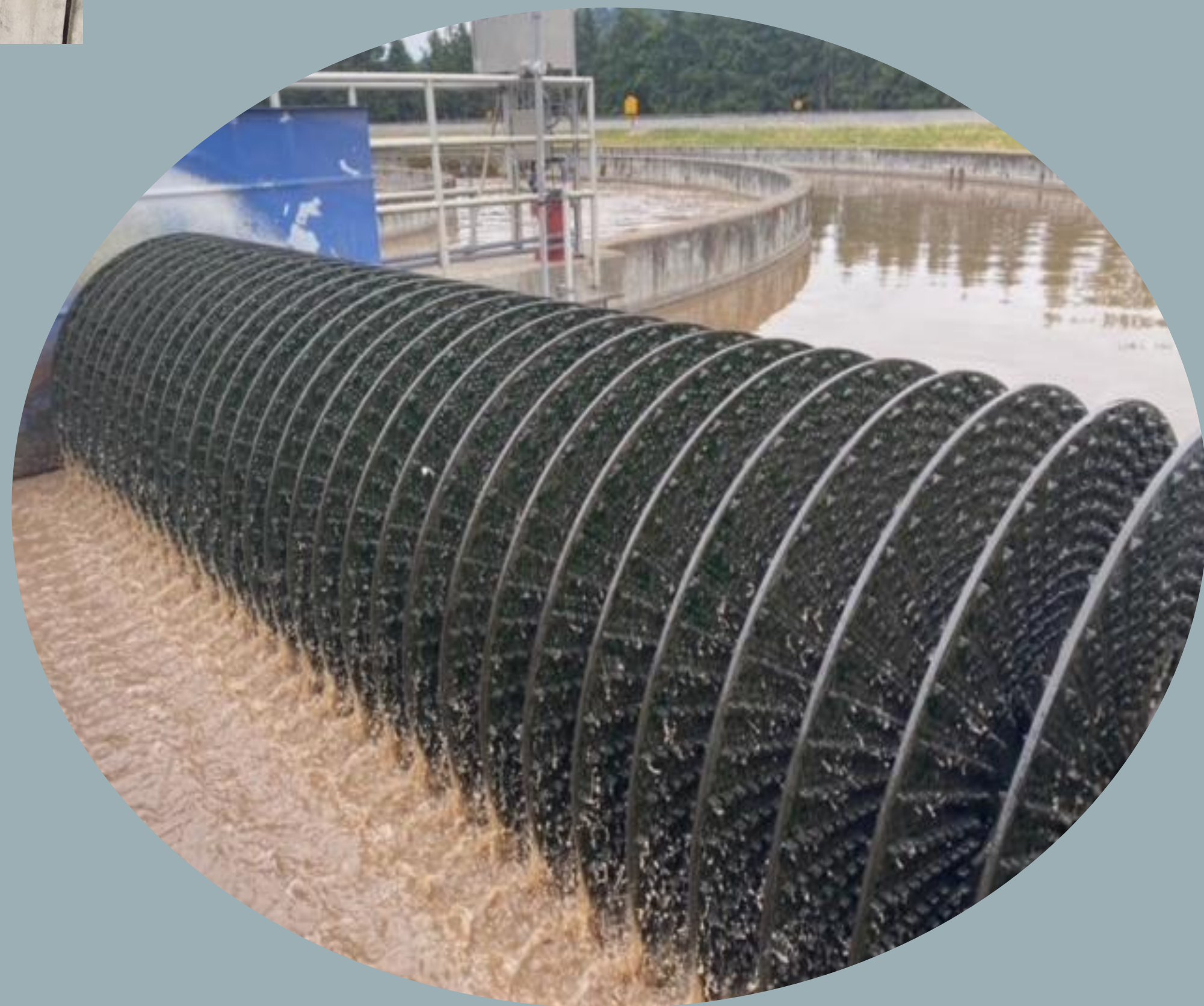
Rotating paddles with aerated disks.
