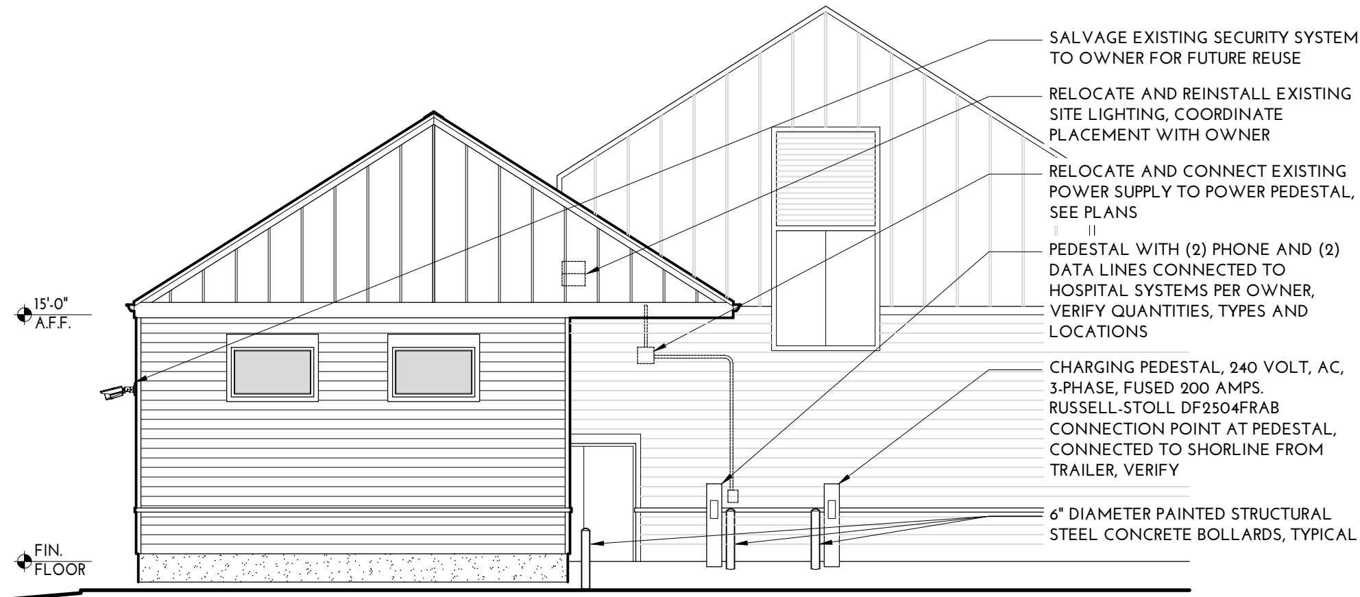
1 A6 SOUTH ELEVATION 1/8" = 1'-0"
